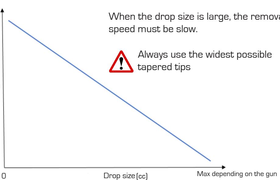
When the viscosity increases, reduce the speed and increase the drawback. When the drop size is large, reduce the speed and increase the drawback. It is important to adapt the diameter of the tapered tips preferably G14, depending on the viscosity of the fluid, in order to allow a good flow and to obtain a clear cut after the dose.
