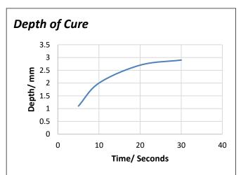
Graph shows the depth of cure at 25 mW/cm² and 405nm. The depth of cure will depend on the power of the UV lamp, its spectral output, the distance between the lamp and the adhesive.
