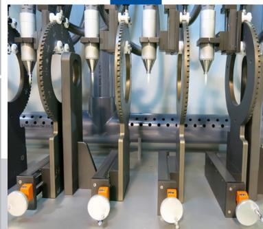
**3DT manufactures a complete line** of highly reliable, innovative corona and plasma surface treatment systems. Our systems improve adhesion on a wide array of plastics, composites, cardboard, rubber, foam, glass, and metal.
