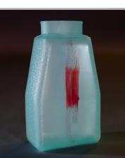
Note the improved adhesion of dyne solution in the treated area.
