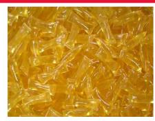
Polyolefin hot melt adhesive of the latest generation
