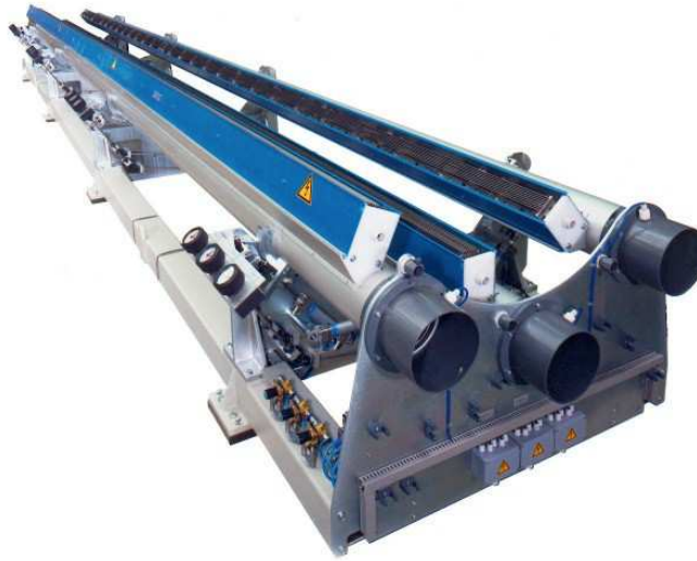
Fig. 11 6m BOPP station with 3 electrode assemblies
