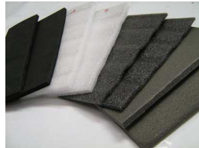
Fig. 19 Multiwall and foam materials treatable with Linear Plasma
