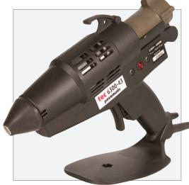
Extremely robust 43mm (1¾") spray glue gun with power on light. Designed for industrial use, it sprays hotmelt at any angle with adjustable spray pattern. Cover large areas with a non-toxic adhesive spray system. Apply hotmelt to heat sensitive substrates without damage. 8 bar (120psi) 85 l/min (3 cfm) air supply required.
