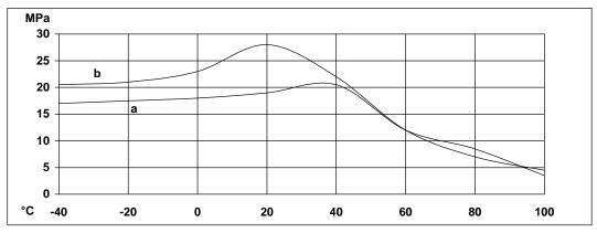
Roller peel test (ISO 4578) Cured 16 hours/40°C 5 N/mm
