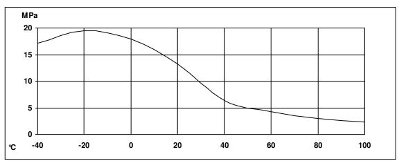
Roller peel test (ISO 4578)
