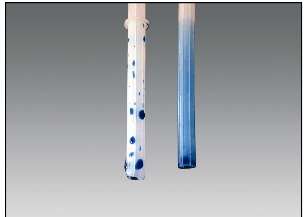
Before and after TubeDyne treatment. Note how the dyne solution wets-out after treatment.
