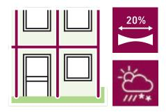
SP510 is a low modulus sealant and is low slump even in warmer temperatures. It has excellent application properties. It cures with air humidity, to form a tackfree surface and provides good resistance to light, ageing and weathering. SP510 is suitable for long term elastic sealing of window and door perimeter joints and movement joints between construction components. It can be used for indoor\* and outdoor applications. It is compatible with metals and most construction materials.
